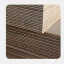
Pin block: 19 cross ply hard maple; High tightness for tuning pins.
